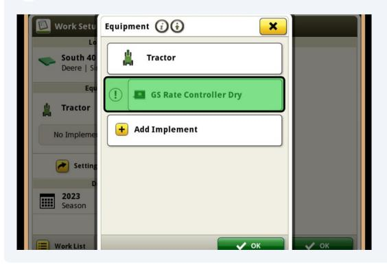
If a Setup File has not been loaded to the display with an applicable implement, Operator will need to add one. Click "Add Implement" at bottom of the screen.
