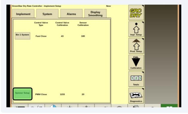
6 Similar to the Conveyor/Apron Control Valve, the Spinner Control Valve will ask for calibration numbers that can be found in the Operator's Manual of the Implement
