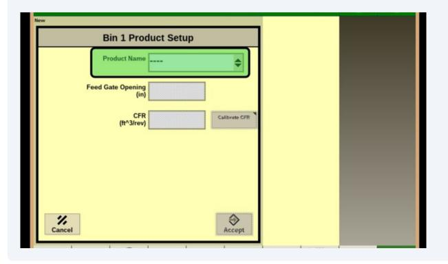
Enter the Feed Gate Opening in Inches as well as the CFR. CFR is the Cubic Feet per Revolution. CFR is generally found in the Operator's Manual of the implement. This will change based on the Gate Opening
