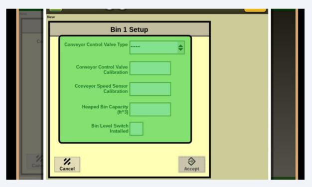
After filling out the information for the Conveyor/Apron Control Valve, select "Spinner Setup" to setup the system controlling the spinners
